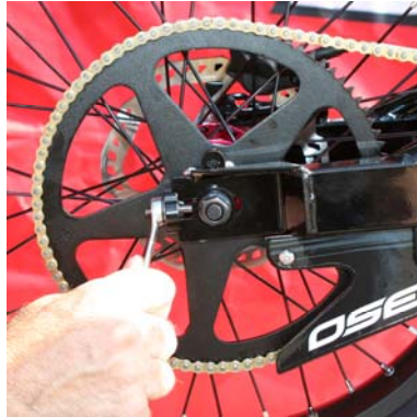
Chain tensioner nut (10mm).
