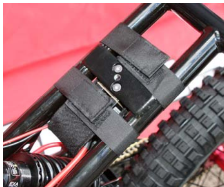
Relay in a Velcro bag.
